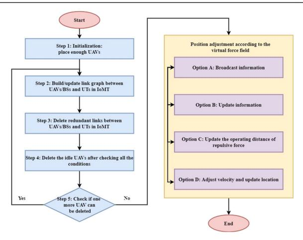
Fig. 5 Flowchart of Unified Greedy Quest Algorithm for Internet of Medical Things (UGQA-IoMT) algorithm
